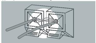
• Stripped cords are touching each other due to excessive removal of insulation.
